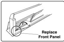
Replace the front panel by hooking the lower front edge of the front panel over the lower front edge of the ventilator.
